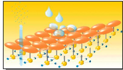
**Effect:** As **DeepSeal 50** is a unique combination of Silanes / Siloxane and Acrylic liquids. Surfaces treated are not only water repellent but also sealed against penetration of rainwater under wind pressure and against most other staining materials such as motor oils, red wine and mild food acids. **DeepSeal 50** highlights the natural colour of masonry but does not produce a glazed finish. However over application will produce a “wetted” effect and a subdued glaze to the surface.
